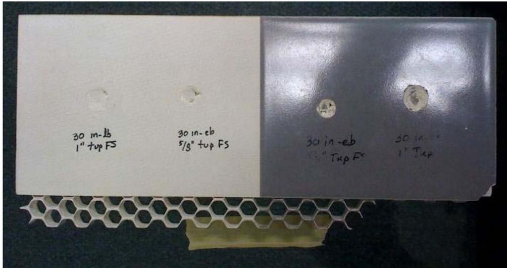
Figure 15: Honeycomb CMC Sample
