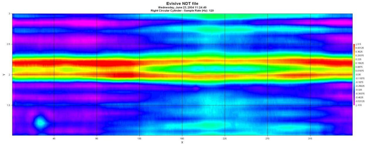
**Figure 19: Evisive Scan image of an unacceptable HDPE Thermal Butt Fusion Weld (flaw is lack of fusion from 150 to 200 °)**
