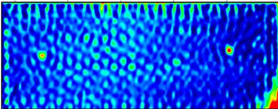
Figure 16: Evisive Scan of the Honeycomb CMC Sample
