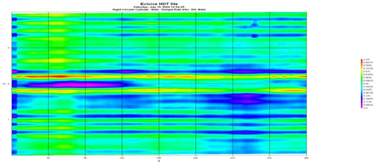
**Figure 20: Evisive Scan image of an unacceptable HDPE Thermal Butt Fusion Weld (flaw is lack of fusion due to uneven assembly pressure)**
