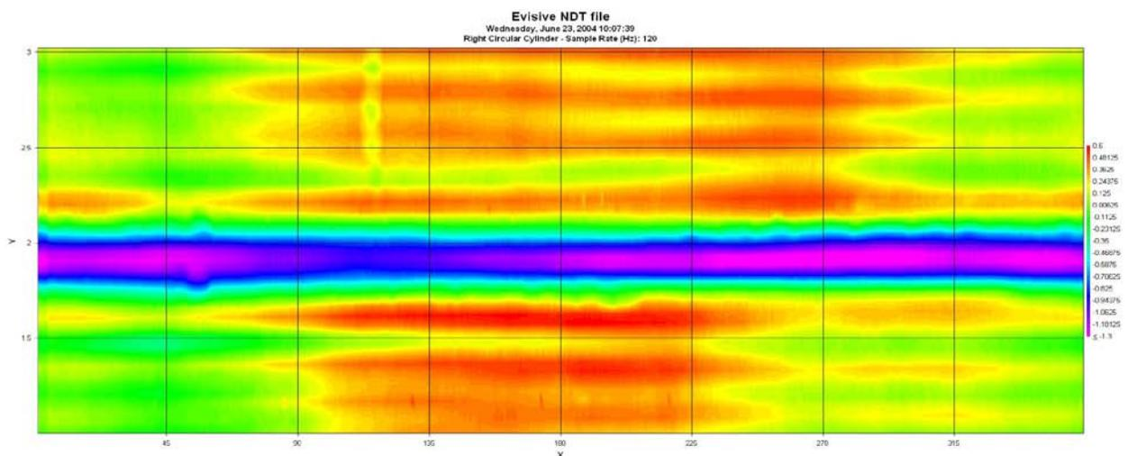
**Figure 18: Evisive Scan image of an acceptable HDPE Thermal Butt Fusion Weld**
