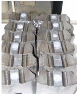
Figure 8 – Tensile Test Result Joint 2 Sections
