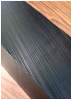
Figure 2. Close – up of HDPE Block Fusion Zone
