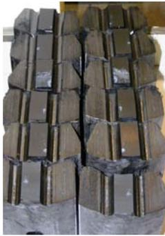
Figure 7 – Tensile Test Result Joint 1 Sections
