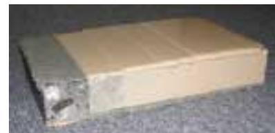
Figure 8. Concrete block with application of varying thicknesses of polyurea coating.
