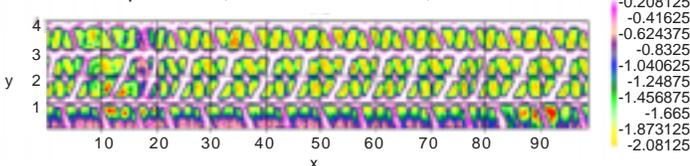
Figure 11. Microwave scan of same passenger tire with intentionally induced defects at X = 10 and 90 degrees.
