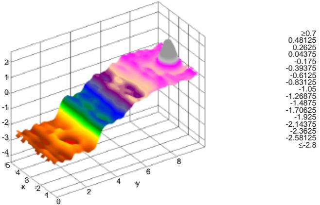
Figure 9. Microwave NDE scan of polyurea coated concrete showing response to varying thickness of coating. Note rebar indications (conical and circular features) at top and bottom of scan.
