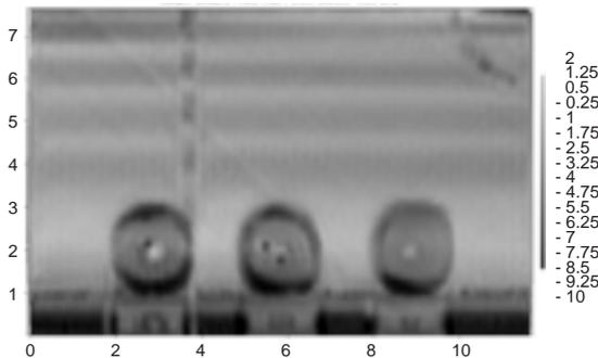
Figure 6. Microwave NDE scan of rotor, front side. Note interior details such as spar (vertical line) and open cell (right upper corner).
