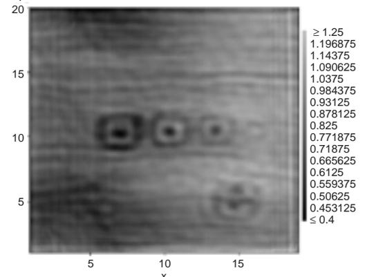
Figure 14. Microwave NDE Scan of Spray On Foam Insulation coupon showing internal defects.
