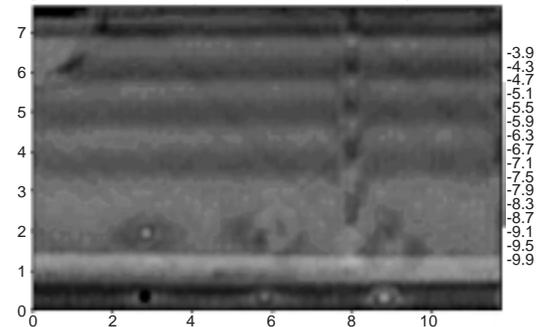
Figure 7. Microwave NDE scan of rotor, back side. Defects visible from reverse side as well as spar and open cell (reversed positions from figure 6).
