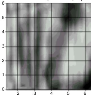
Figure 2. Microwave scan of plywood coupon showing internal and external wood structure.
