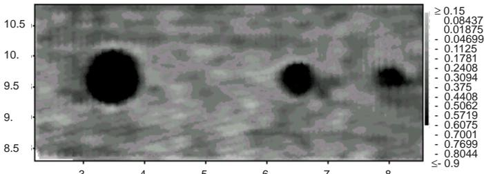
Figure 4. Ceramic coupon (silicon carbide CMC) with three embedded defects.
