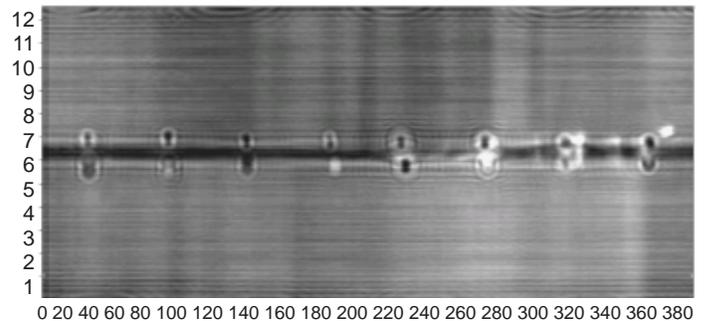
The coupon shown above is a piece of nominal 8 inch (8.5 inch OD) polyethylene pipe, approximately 12 inches long with 8 defects embedded in each side of the thermal fusion butt weld. Note the 1/16 inch by 1/16 inch foil marker at X=0, Y=1.
