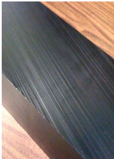
Figure 2 Close-up of HDPE Weld Block Showing Weld Location
