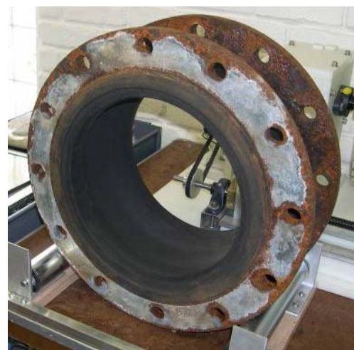
FIGURE 2: EXPANSION JOINT MOCK-UP
